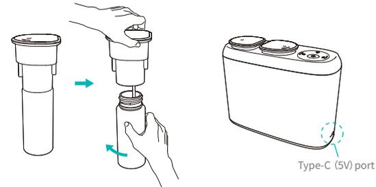
② Unscrew the essential oil bottle in the direction of the arrow, add the essential oil supplies and put it back into the atomizer head.
